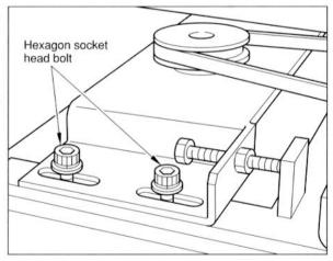
Tighten the adjuster bolts evenly on the right and left sides of the motor bracket and adjust the belt tension correctly.
