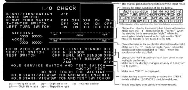
If the handle or the accelerator is not properly adjusted, make necessary adjustments, referring to "7—4 Replacing and adjusting the volume knobs" on pages 33 to 34.
