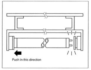
It is recommended that the glow lamp should be also replaced.
