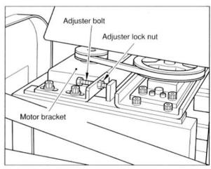
Loosen the hexagon socket head bolts (4 pcs.)fastening the motor bracket and remove the belt.
