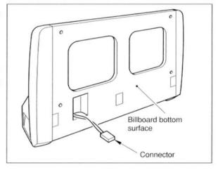
Lift the billboard and connect the connector to the projector unit side. Fasten the billboard with the screws removed in step 10, being careful not to catch the bound wires.
