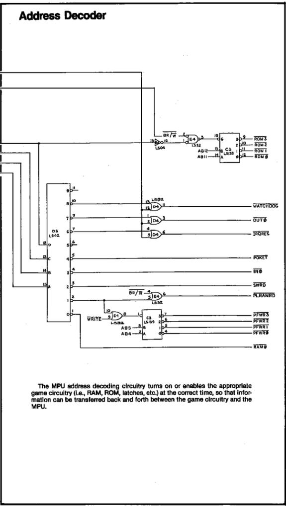
The MPU address decoding circuitry turns on or enables the appropriate game circuitry (i.e., RAM, ROM, latches, etc.) at the correct time, so that information can be transferred back and forth between the game circuitry and the MPU.
