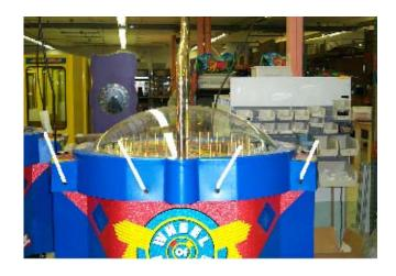
Lift the cover up to access the Display P.C. Boards.
