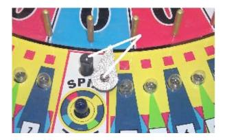
Remove the Light Ring graphics by lifting the ring up.
