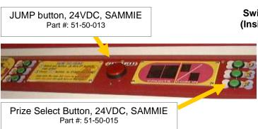
Switch & Meter Bracket (Inside of the Coin Door)
