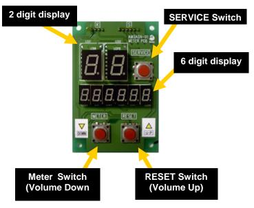
Switch & Meter Bracket (Inside of the Coin Door)
