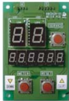
METER PCB AM3AGN-01 Part#: 51-20-215
