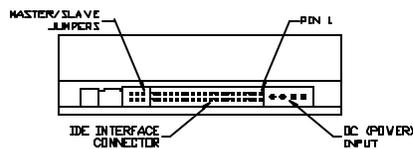
FIGURE 5 – REAR VIEW OF STANDARD CD-ROM DRIVE
