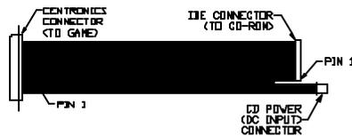
FIGURE 4 – CENTRONICS/CD-ROM INTERFACE RIBBON CABLE
