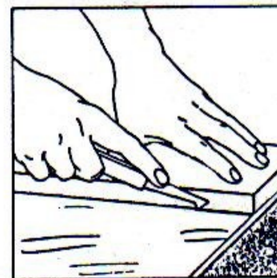
Always draw the scribing knife along a straight edge.
