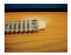
8- Slide the slide mechanism out of the groves in the mechanical nose assembly. Now remove these two screws in the slide mechanisim detaching the banding from within the mechanical nose assembly.
