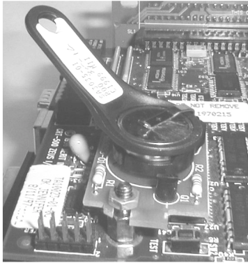
FIGURE 18 - ADAPTER BOARD AND KEY INSTALLED
