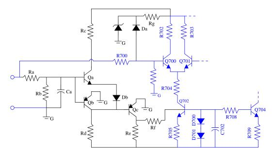
Figure 7: P314 input protection PCB half circuit
