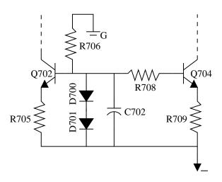
Figure 4: WG K6100 X deflection amp bias circuit
