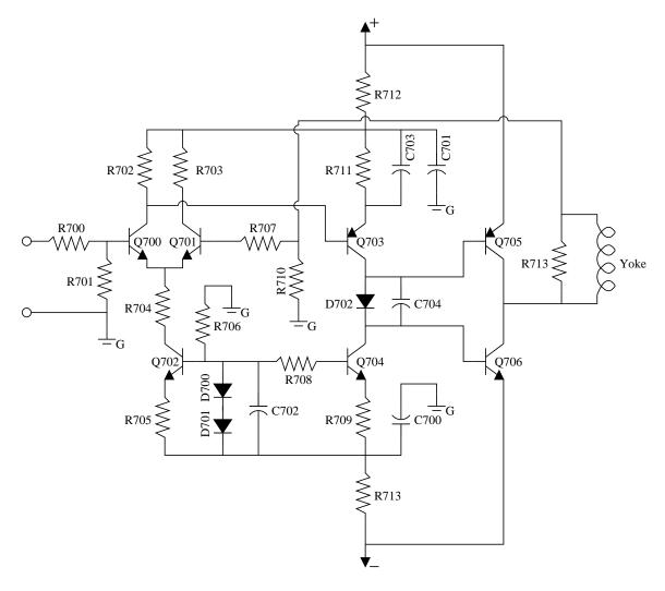
Figure 3: WG K6100 X deflection circuit
