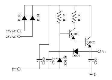
Figure 1: WG K6100 low voltage power supply
