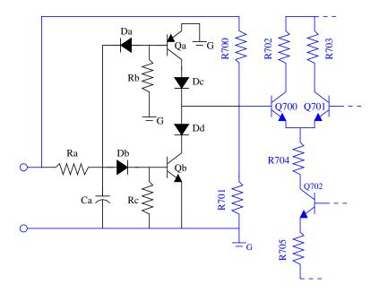
Figure 8: P327/P339 input protection half circuit
