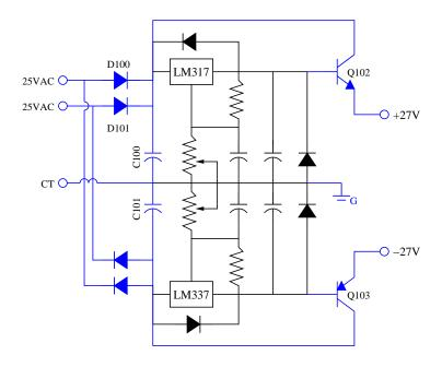
Figure 2: WG K6100 replacement low-voltage regulator
