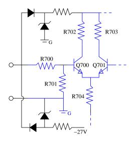
Figure 6: Frank the Crank's Zener diode input protection mod
