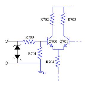
Figure 5: Atari Zener diode input protection mod
