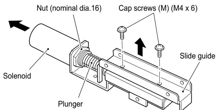
7. Pull out the solenoid plunger, taking care not to lose the spring.
