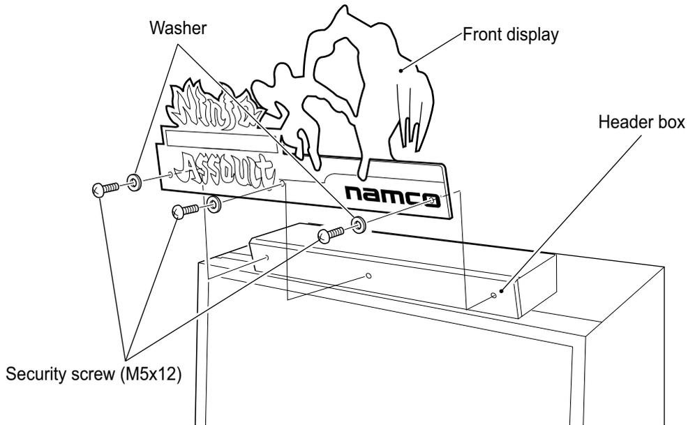
2. Remove 4 off security screw and remove the Front Panel from the Header Box.
