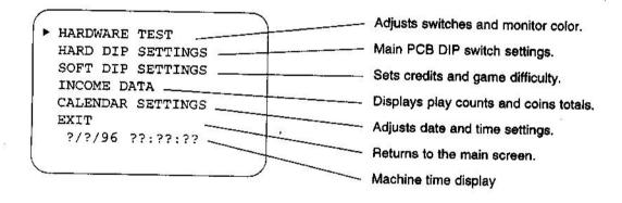
3. Hardware test (If software is not loaded, only the HARDWARE TEST mode can be used.) Carries out the various cabinet checks.
