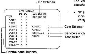
The various switches on the control panel and elsewhere can be checked.
