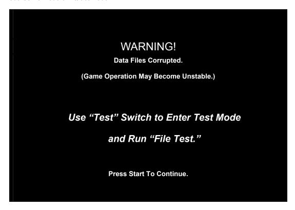
**CORRUPT FILE SCREEN.** If you see the above screen, your VGM computer has corrupt files. To determine which files are corrupt, you can run the File Test. (See *Chapter 3, Audits, Adjustments & Diagnostics.*) The File Test can't repair corrupt files, though. The only solution is to perform a system recovery.
