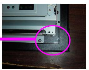
Sandwich plastic cover between the monitor frame and 32" LCD Monitor then tighten a screw (Pan Phillips 8-32x 5/8)
