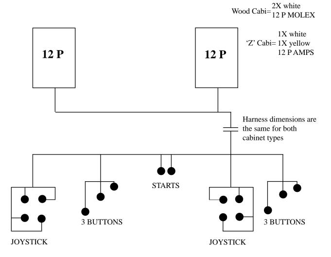
Each " • " has a switched wire and a white logic ground return with slip on solderless connectors.
