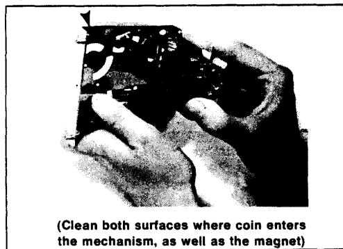
Figure 3-4 Surfaces to Clean Inside the Coin Mechanism
