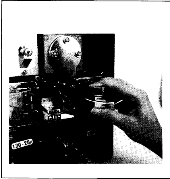
Figure 10 Hinging Open the Magnet Gate Assembly
