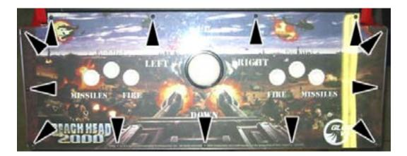
2. Next remove the 6 buttons from the control panel shown by the arrows in the picture below. You will need to keep 4 micro switches with buttons as these will be re-used again with the joystick configuration.
