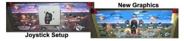
3. Install two buttons on either side of the joystick as shown by the arrows with letters on top in the picture below. Arrows with the letter "C" are for the Canon buttons; Arrows with the letter "M" are for the Missiles buttons. The missiles buttons are wired with the Green wire coming off the joystick, canons use the Grey wire.
