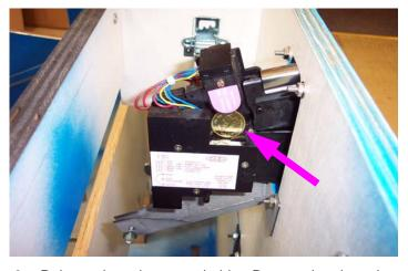
Release the coin sensor holder. Be sure that the coin or token is properly seated.
