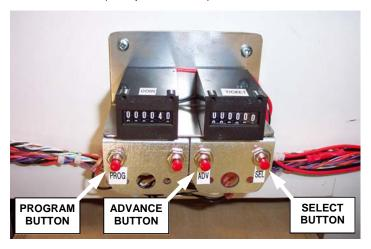
3. To enter programming, press the Program button once. Each programming mode is identified by the "lock lit" (mode 1, 1st lock light, mode 2, 2nd lock lit; etc.). To exit programming, press the Program button once.
