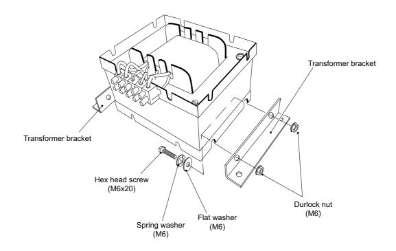
7. Refit the new Transformer using 2off hex head screws (M6x20), with flat and spring washers, and 2off wood screws (No10x³¼).
