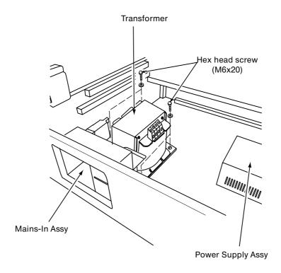
6. Fit the Mounting Brackets(supplied) to the Transformer with 4off hex head screws (M6x20), flat and spring washers and Durlock nuts (M6) (supplied), as shown below.
