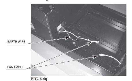
Also, use LAN joints to connect the LAN cables.
