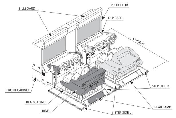
FIG. 4a Overall Diagram
