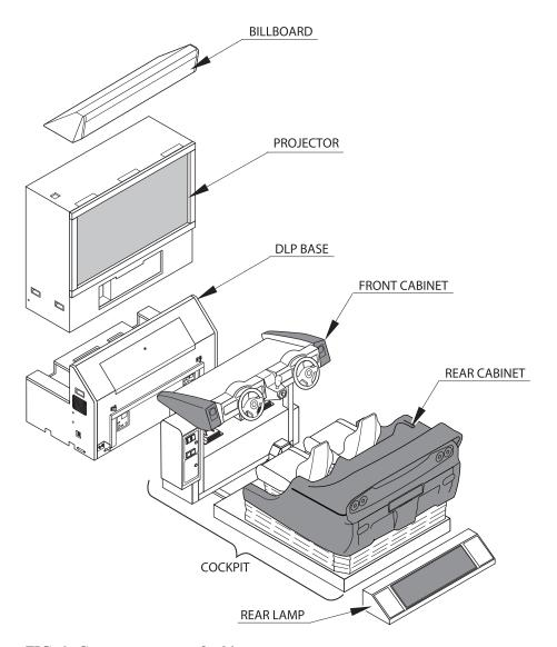
FIG. 6a Component parts of cabinet
