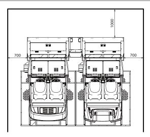
FIG.2 Operation Area (Unit: mm)
