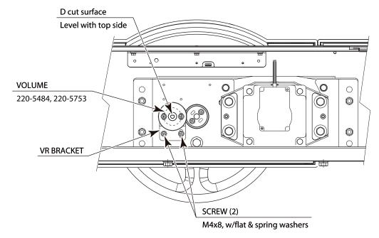
FIG. 9-1d STEERING WHEEL MECHANISM VOLUME
