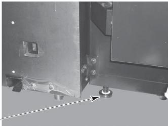
FIG. 6-8a Ground adjusters
