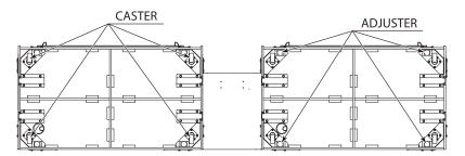
FIG. 6-54d Bottom view of two DLP bases joined together
