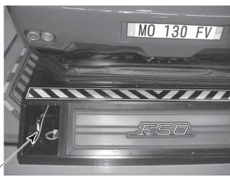
Draw the wiring and the earth wire inside the rear lamp.
