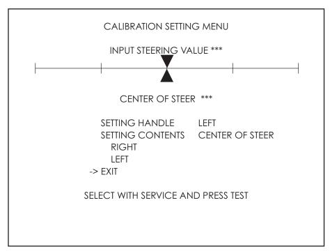
FIG. 6-13d CALIBRATION SETTING MENU Screen
