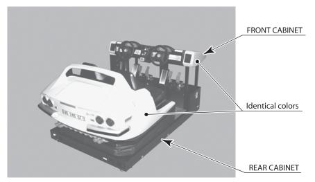
FIG. 6-6a Match the color of the front cabinet and rear cabinet
