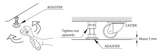
FIG. 6-5e Adjustment of adjusters
