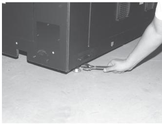
FIG. 6-5c Ground adjusters
