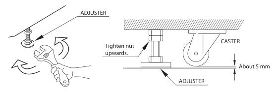
FIG. 6-8c Adjust the adjusters
