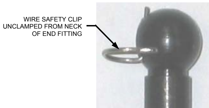
FIGURE 2 – CLOSE-UP VIEW OF THE END OF THE GAS SPRING
