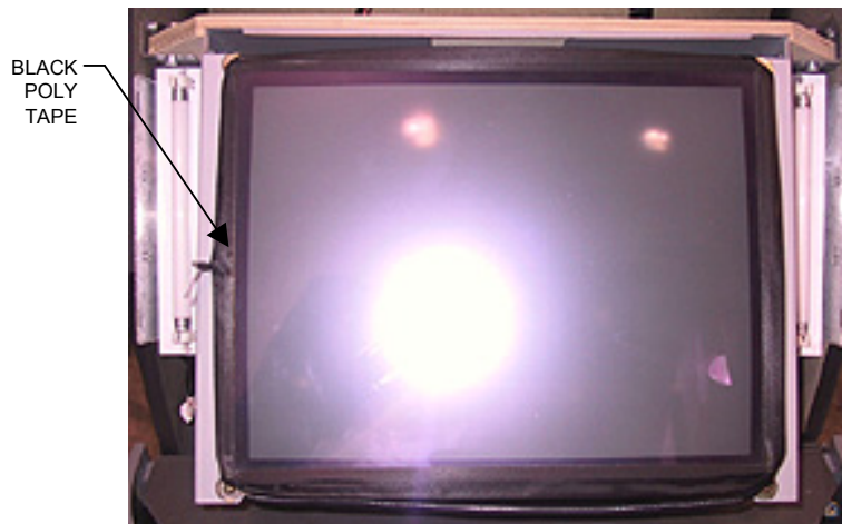
FIGURE 20 - MEGATOUCH COMBO JUKEBOX - MONITOR AND TOUCHSCREEN
