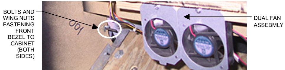
FIGURE 18 - MEGATOUCH COMBO JUKEBOX - INSIDE REAR OF CABINET
