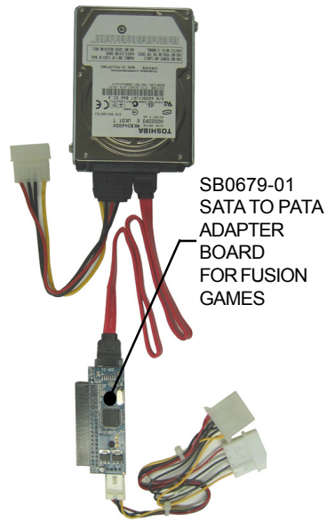
FIGURE 6 - NEW SATA HARD DRIVE ASSEMBLY FOR FUSION GAMES WITH ECS MOTHERBOARDS (SEE FIGURE 9 FOR CONNECTIONS)
