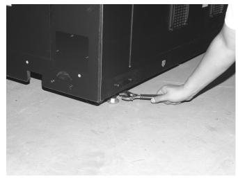
FIG. 6-4c Ground adjusters
