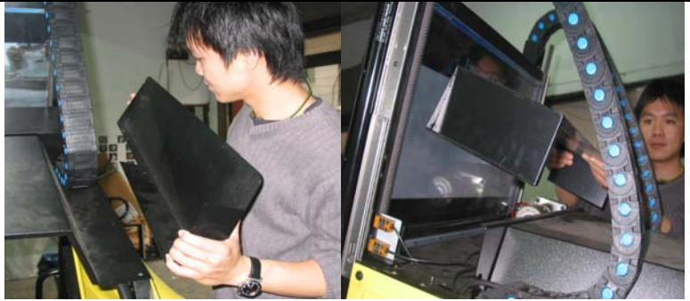
(b) While Monitor is at Up position, the LED light on sensor (4+OT) is off but LED light on sensor (4-OT) is on, which is correct.
