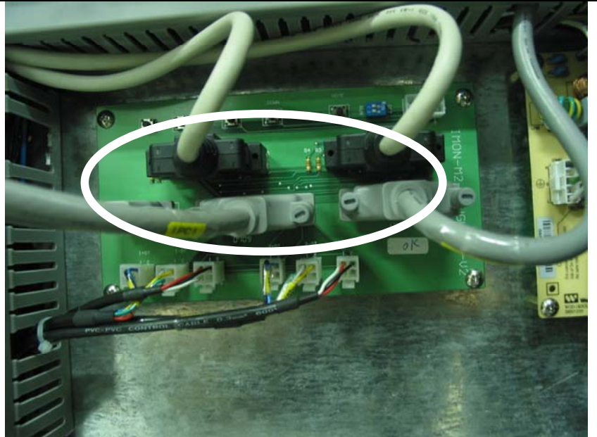
(b) Check Servo Amplifier Connector (CN2) is well-connected.
