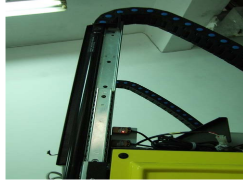
(b) Loose the screws which fix the sensor
