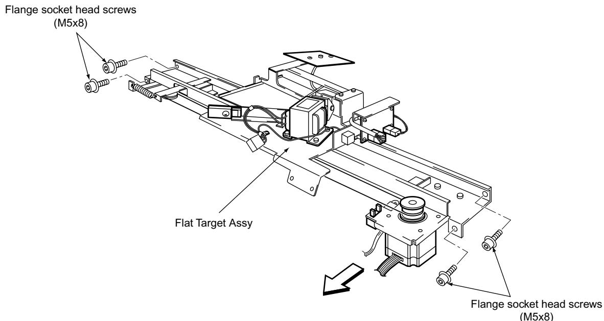
5. If the Target needs adjusting, bend downwards by placing a thumb underneath the rear of the target and pressing down at the front.
