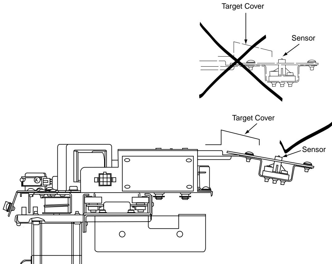
The Upper and Lower Target Assemblies are different.
