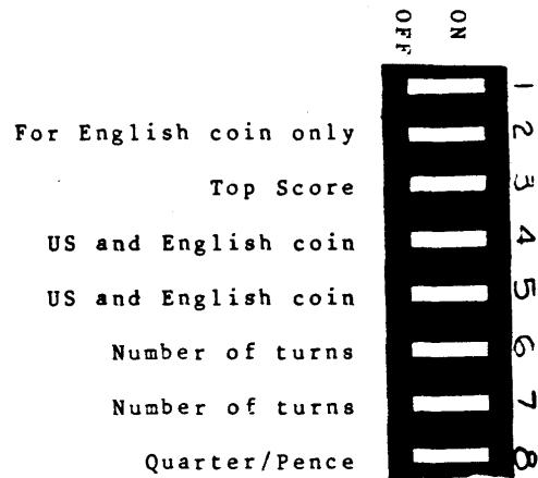
Figure 6.5: Functions of the 8-position DIP Switch
