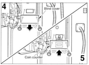
Reconnect the coin counter connector to the counterpart inside the machine.
