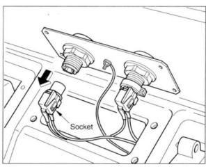
4 Loosen the nut and remove the press-button.
