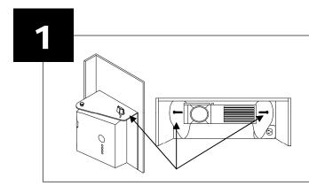
Projection is pre-adjusted at the factory but minor adjustments may be required. (1) Vertical adjustment (Tilt) To center the image horizontally on the screen, loosen the large knob on both sides of the projector and tighten it when it is adjusted properly.
