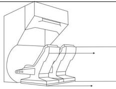
Lift the seat module using the 2" 1x2 metal tubes as handles until the back of the seats touches the floors (fig C)
