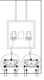
IMPORTANT: When reinstalling the plates, slide them toward the outside of the machine.
