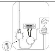
Unbolt the seat module from the main cabinet Slide the seat module a foot away from the main cabin (being careful not to damage the seat cables)
