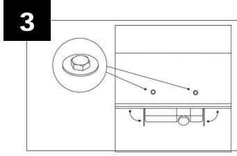
Horizontal Adjustment: To rotate the projector find the two adjustment bolts at the top of the machine (pictured here) loosen them, adjust view then tighten.
