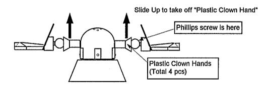
3) Remove 4 Phillips of screws on top and loosen 4 pcs of bottom to take off "Plastic Clown
